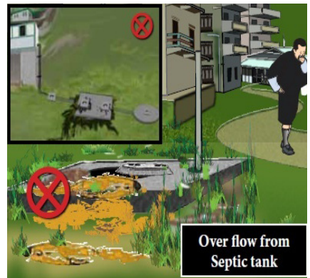
Figure 9. Sewage overflow from septic tank
