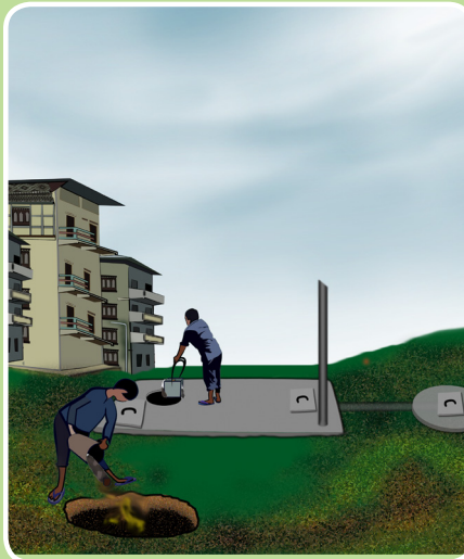
Safely dispose of sludge manually if cesspool services are unavailable
