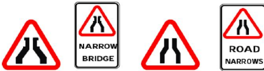
Figure 12: Road width signs
