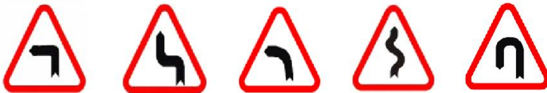
Fig: 10 Horizontal Alignment sign
