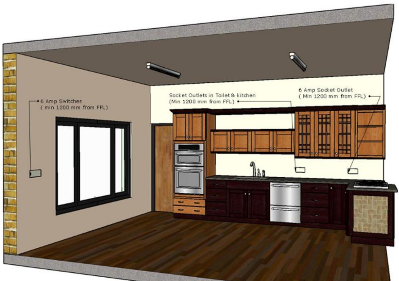
Figure 2.6: Standard height of electrical fittings in kitchen
