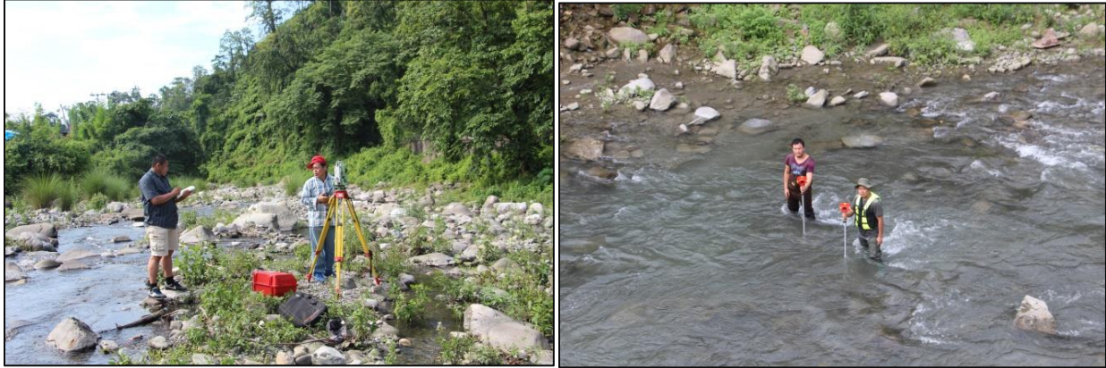
Figure 12: Cross Section Survey being carried out (Left and Right)
