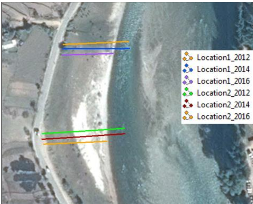
Figure 24: Google image showing the erosion at the right bank of Mochu in a span of 2 years (2014 and 2016)
