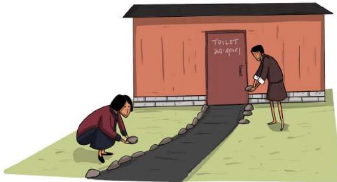
Figure 7: Lay guide rocks and colour the guide rocks to help person with partial vision impairment
