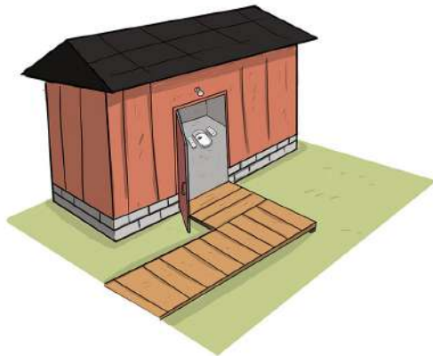
Figure 1: Ensure flat landing (size of the flat landing/platform should be 5ft x 5ft) between the ramp and the toilet entrance (not even small steps at the toilet entrance or lips at the end of the ramp).
