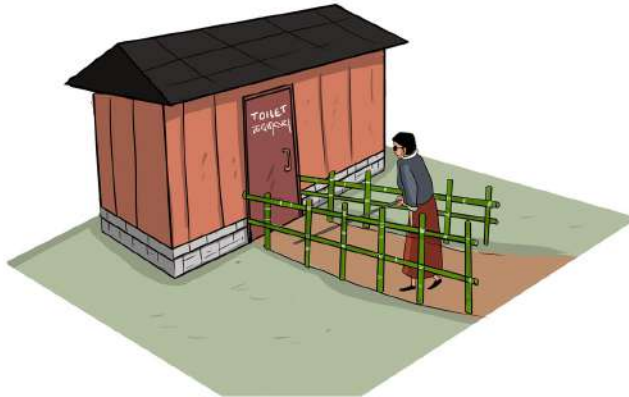
Figure 5: Bamboo/Iron rail throughout the pathway with no obstructions. The height of the handrail should be 2ft 6 inches – 3 ft) above the ground
