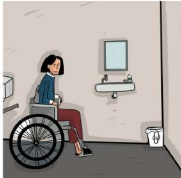
Figure 1: Install tap points inside the toilet with soap. Remove any obstacles leading toward the tap station so wheelchair user can wheel in under the space. The height of the tap stand should be 2ft 10 inches.
