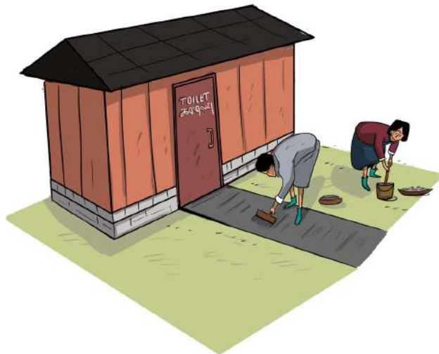
Figure 3: Building anti-skid slabs (Use cement, gravel or rubber etc to make the footpath antiskid by adding etchings/hatchings) throughout the pathway.
