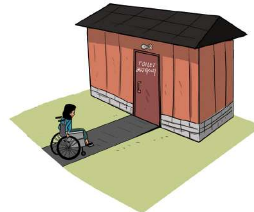
Figure 4: Build accessible path with low gradient ramp/pliable gradient (Slope of the ramp should be 1:15 (1 ft height for every 15 ft) and ensuring 3feet footpath width minimum.
