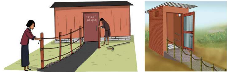
Figure 6: Alternatively use guiding rope with no obstructions for persons with vision impairment. The height of the guiding rope should be 2ft 6 inches – 3 ft) above the ground. Consider provision of white cane/stick
