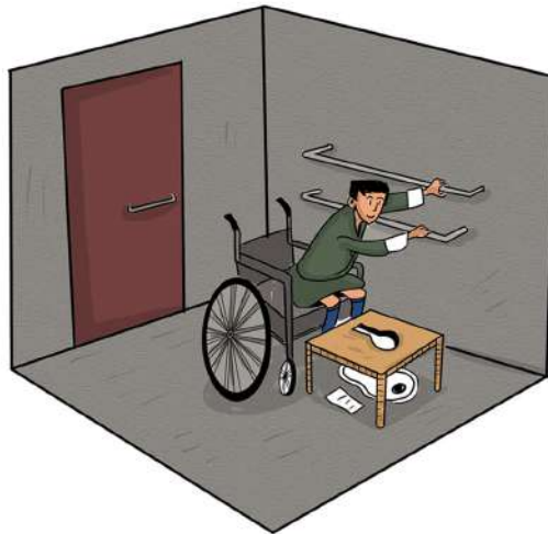
Figure 5: Use pedestal/commode chairs/ wooden seat etc in case replacement of squatting pan is not possible
