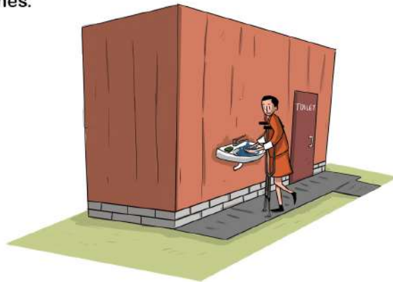
Figure 2: If tap point inside is not feasible, install handwashing station near the toilet. Remove any obstacles leading towards and below the tap points. Ensure all household members keep/replace soap in agreed location
