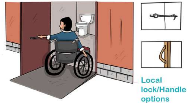
Figure 2: Install easy locks/handles on doors (e.g. Simple traditional wooden latches and metal hook options that is easy to use). Place the door latch from inside and handle from outside are at 2 feet 6 inches height from the floor.
