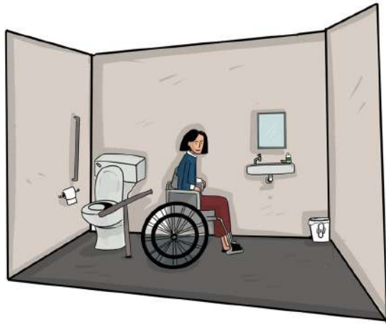
Figure 3: Provide sufficient room size (at least 8ft x 7ft) for wheelchair mobility in the toilet. Place waste disposal (Pad) bins with lid/cover
