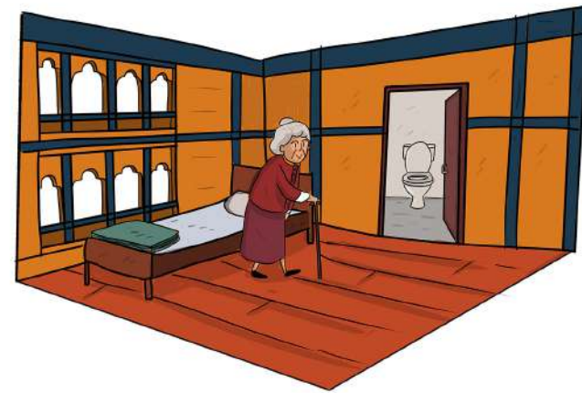
Figure 2: If the house structure permits, build toilet inside the house. Ensure to remove batten (between the room and toilet) to improve accessibility, and maintain slope for flow of water on the floor towards the drainage pipe.
