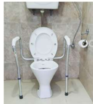
Figure 1: Use European pot (sitting) instead of the Indian ceramic pan. Install/fix grab bars and rails on the floor/wall (Grab bar height should not be more than 2 ft 6 inches).
