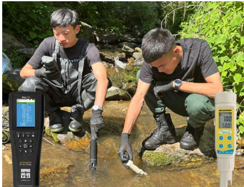
Figure 2. 2: YSI ProDSS Multiparameter Water Quality Meter and PCS Testr used for water quality measurement
